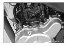
• Attach the timing light [A] to the central ignition coil lead in the manner prescribed by the manufacturer.
