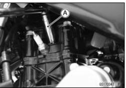
• Insert the spark plug vertically into the spark plug hole with the spark plug installed in the plug wrench [A], and finger-tighten it first.
