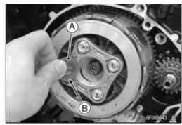
• Using the primary gear holder [A], hold the clutch housing gear and primary gear.
