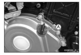
• Remove the oil strainer cap [A] from the bottom of the engine.
