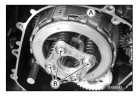
• Install the washer [A] so that the chamfer side [B] faces outside.
