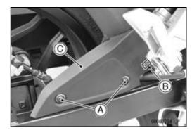
• Remove the mud guard bolts (front) [A] and collars.
