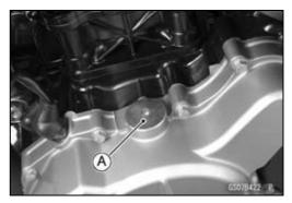
Turn the camshaft clockwise, and align the "T" mark [A] on the alternator rotor with the projection [B] on the alternator cover.
