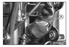
• Slide the dust cover [A], and disconnect the starter lockout switch lead connector [B].
