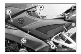
• If necessary, remove the mesh cover [A] by removing the screws [B].
