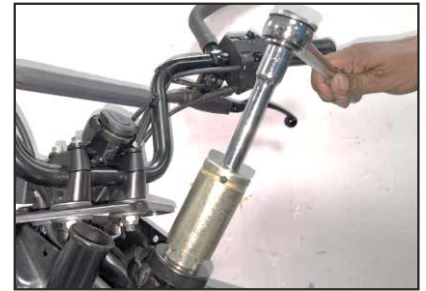
Balancer lock nut loosening & tightening tool for steering slotted nut
