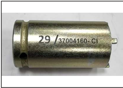
Balancer lock nut loosening & tightening tool for steering slotted nut
