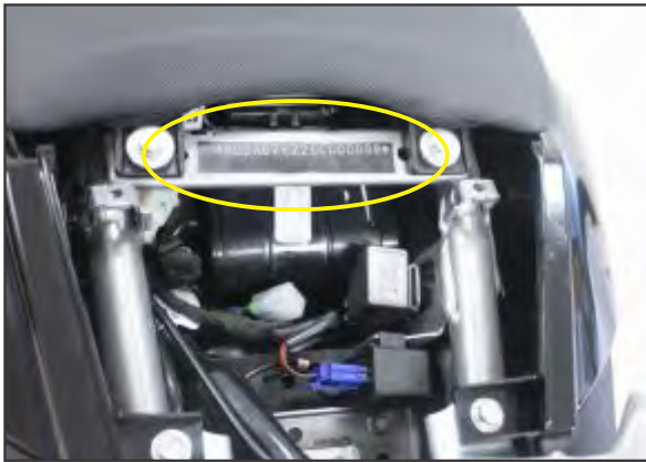
▶ Frame Number Location On Seal Lock Mounting Bracket (Alpha-Numeric - 17 Digits)
