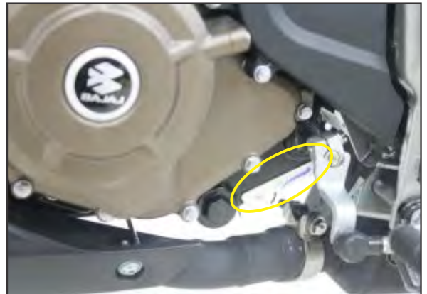
Engine Number Location On LH Side Crankcase Near Gear Change Lever (Alpha-Numeric - 11 Digits)
